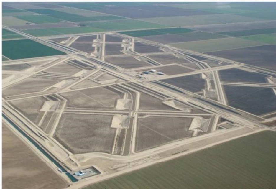
Figure 3.2 Constructed Spreading Ponds for Groundwater Recharge (SemitropicWSD).
